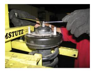
5d. Install your required spacers for the desired height on the BELLTECH Lifting & Lowering Shock.
