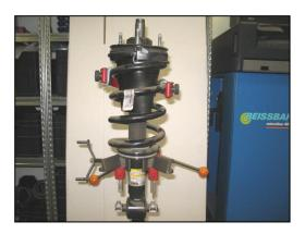
5b. Using an open wrench, remove the top mount.
